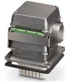
Panel feed-through set (panel mounting base, stackable housing, 2 contact inserts, housing cover)
